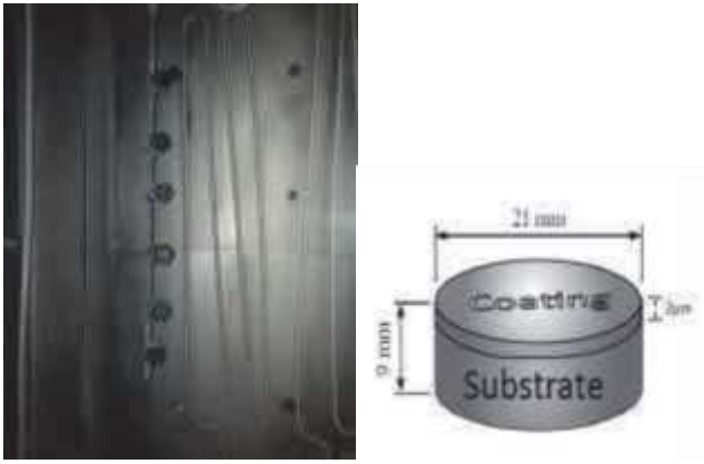
Fig. 3 The Samples placed in the surface coating vacuum chamber and the size of the Samples
